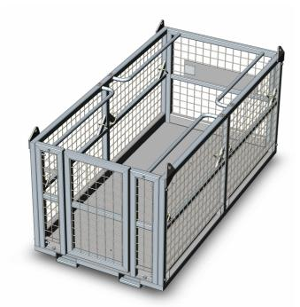
The type WP-2 Crane Cage Work Platform has been designed strictly in accordance with Australian Standard AS 1418.17 and is suitable for a maximum of six people. Work performed in this Cage shall be limited to special tasks of short duration in situations where necessary to elevate personnel where it is not practicable to erect scaffolds or use a specially designed device. Fork Arm slippers are provided for transport purposes only. The standard finish on the Cage is Zinc finish.
