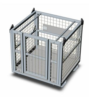
The type WP-1 Crane Cage Work Platform has been designed strictly in accordance with Australian Standard AS 1418.17 and is suitable for a maximum of four people. Work performed in this Cage shall be limited to special tasks of short duration in situations where necessary to elevate personnel where it is not practicable to erect scaffolds or use a specially designed device. Fork Arm slippers are provided for transport purposes only. The standard finish on the Cage is Zinc finish.
