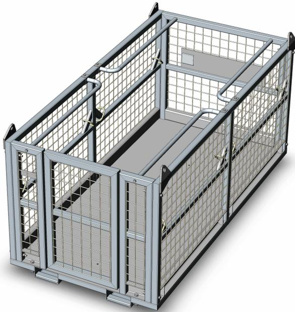
The type WP-2 Crane Cage Work Platform has been designed strictly in accordance with Australian Standard AS 1418.17 and is suitable for a maximum of six people. Work performed in this Cage shall be limited to special tasks of short duration in situations where necessary to elevate personnel where it is not practicable to erect scaffolds or use a specially designed device. Fork Arm slippers are provided for transport purposes only. The standard finish on the Cage is Zinc finish.
